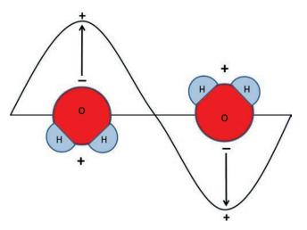
Figure 3 Electric dipole rotation. (Miramar Labs, Inc.)
