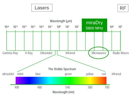
Figure 2 Electromagnetic spectrum with location of microwaves. (Miramar Labs, Inc.)
